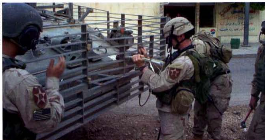
RPG-7-grenade stuck in a Slat Armour of a Stryker IFV
